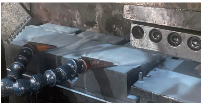
OSG's rack dies are designed to eliminate the machine adjustment often required in die set up.
