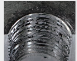
Figure 2. An example of galling.
