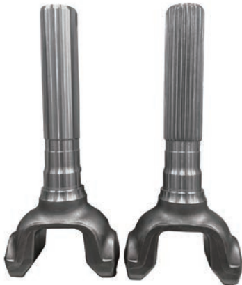
From left, steel spline yoke before and after processing by rack dies. After machining, splines are formed on the shaft.
