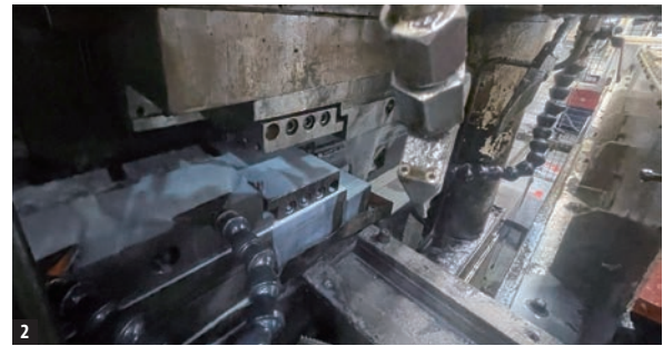
1. Anderso-Cook spline rolling machines are used for the processing of spline yoke made of steel.
