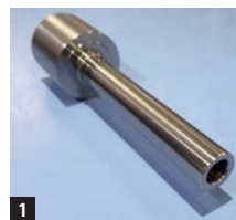
1. A pistol barrel made of ASTM 410 stainless steel (JIS SUS410).
