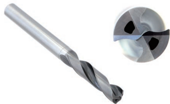
OSG's ADO-SUS series has adopted a tool geometry that emphasizes sharpness to reduce work hardening, thereby prolonging tool life for post-processing including reaming and tapping. Its unique flute form encourages the creation of small cutting chips, which is essential for trouble-free chip evacuation. Furthermore, the ADO-SUS has employed a unique oil hole design "MEGA COOLER" for diameter sizes above 6 mm to suppress heat generation and to facilitate smooth chip evacuation.
