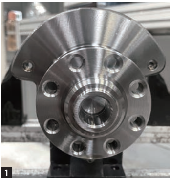
1. Each crankshaft requires the threading of eight M10 x 1 through holes. The drill hole size is dia. 9 mm and 15 mm deep.
