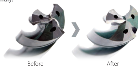
Figure 2. The condition of a 3-flute drill before and after tool reconditioning. With the capability and expertise to bring worn cutting tools back to life for a fraction of the cost of a new tool, reconditioning is highly economical and environmentally friendly.
