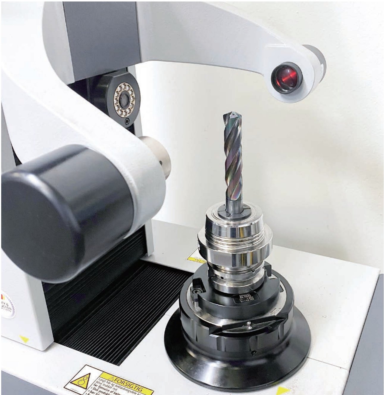
OSG's ADO-TRS 3-flute carbide drill is being presetted at a Zoller tool presetter.
