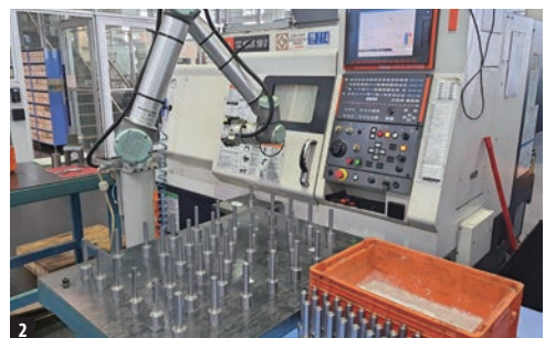
2. The ASTM 410 stainless steel pistol barrels are machined using a Mazak Nexus 150-II CNC turning center. One blind hole at a depth of 55 mm is required to be drilled and reamed per part.
